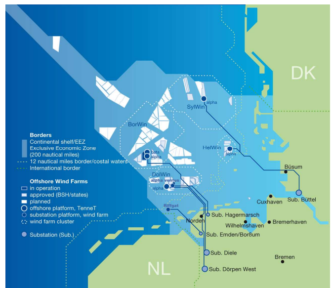
Fig. 1 Geographical division of the planned OWP into four clusters with the allocated transmission routes and NVP in the substations (stand 03.2011)
