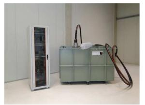
Fig. 1: DRT test system 200kV, 1µF
