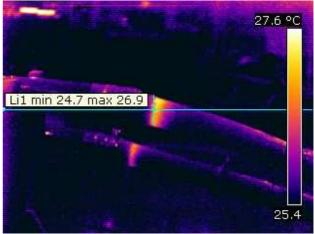
Figure 1 : Stress control heating under nominal voltage
