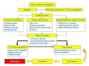
Fig. 2 Process of failure investigation at Liander
