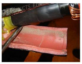
Fig. 1 Example of insufficient installation of a MV joint
