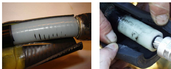
Fig 1: Example of wrong installation work (left) and insulation degradation (right) in a cable accessories. In all these types of insulation defects partial discharges are symptoms.
