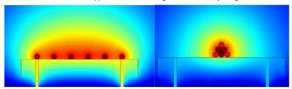
Fig. 1: Examples of FEA of SIWO-KUL™. Six cables are layed on a metallic cable tray.
