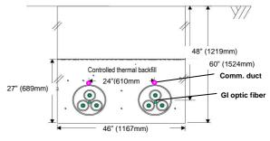
Fig. 1: Typical cross-section of trench
