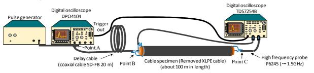
Fig. 1: Measuring setup of the pulse propagation characteristics for the removed XLPE cable
