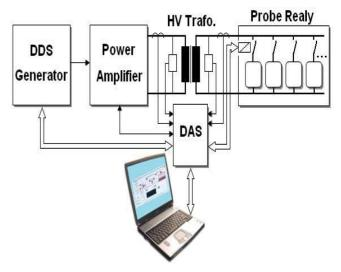
Fig. 1: Block scheme of the ageing test system
