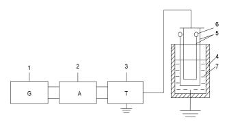
Fig. 1: Setup used for water trees development: 1- Tektronix CFG 253 voltage generator, 2- Amplifier, 3- High frequency transformer, 4- Ageing cell, 5- Samples, 6- Metal balls to avoid discharges, 7- Water/NaCl solution
