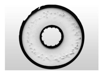
Figure 1: Voids formed on the surface of HVDC cable (Courtesy of M. Kurtz, Ontario Hydro Dobson Laboratories)
