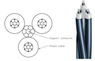
Fig. 1: High Voltage Non-Metallic Screened Aerial Bundled Cable (HV NMS ABC)
