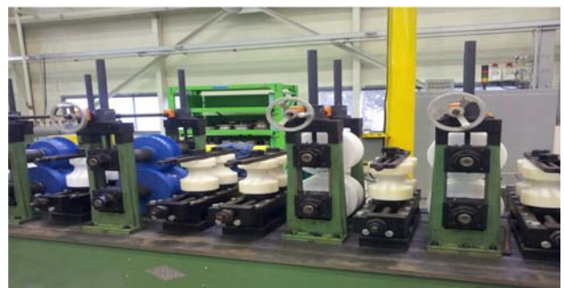
Fig 2. Strip tool for smooth welded metal sheath
