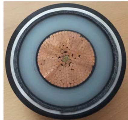
Fig 1. Cables with smooth welded aluminium sheath
