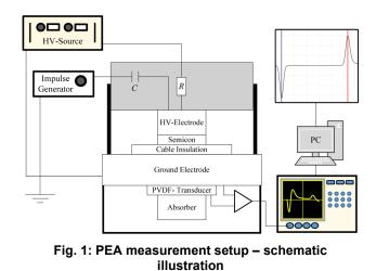
To receive the space charge density  $\rho(t)$  from the measured voltage signal v(t), the influence of the transfer function  $h_{PEA}(t)$  has to be removed.
