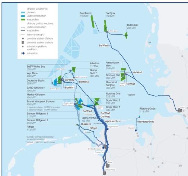
Fig1: Overview of the Offshore Grid Connections
