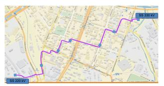
Fig.1. Scheme of laying of cable lines in St. Petersburg.
