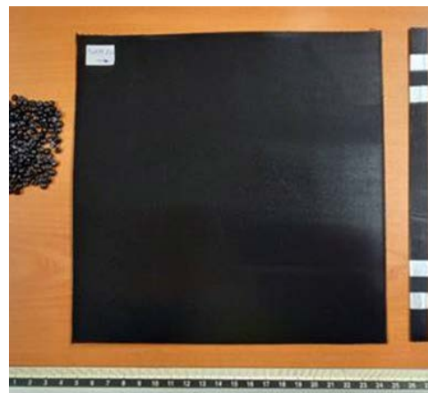
Figure 1 Semicon strip sample obtained from moulded plaque
