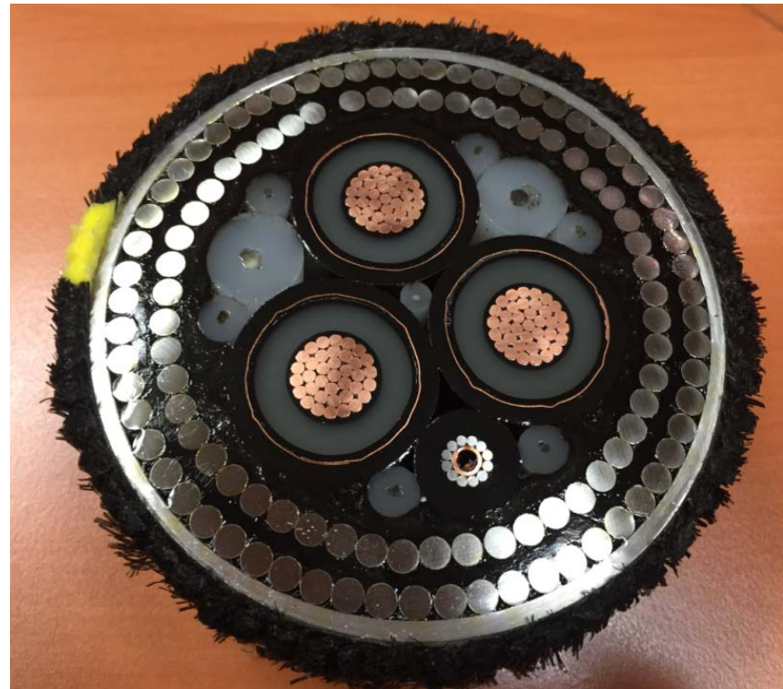
New cable with optical fiber
