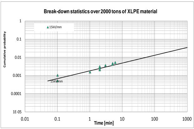
Routine test at15 kV/mm (4 to 6  $U_0$  depending on insulation thickness).
