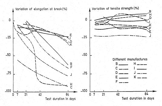
Figure 5c-2. Variation of mechanical properties of XLPE with time at 100°C for a variety of samples from different manufacturers.
