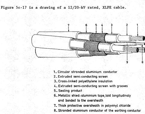
9\_ Earth-conductor lead covering
