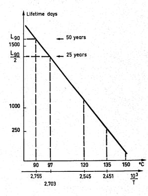
Figure 5c-1. Lifetime for thermal aging of XLPE at various temperatures. This data gives A = 11.47, E/k = 5730 for the constants in Eq. 5c-1.
