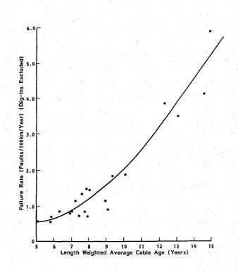
Figure 5f-3. XLPE cable failure rate versus average cable age.
