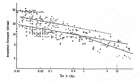
Figure 5e-4. The breakdown strength of XLPE power cables as a function of the loss tangent.
