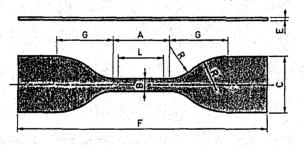
Figure 5c-11. A test bar for mechanical testing of insulation.
