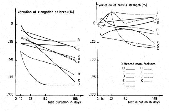
Figure 5c-3. Variation of mechanical properties of XLPE with time at 110°C for a variety of samples from different manufacturers.
