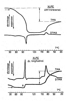
Figure 5c-15. Small-load thermal mechanical and differential mechanical data on XLPE from an extruded cable.
