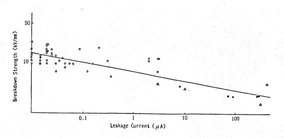
Figure 5e-3. The breakdown strength of XLPE power cables as a function of dc leakage current.
