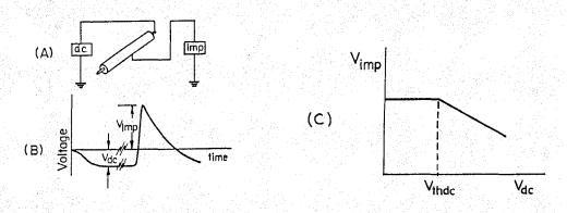
Figure 5e-2. (A) Diagram of circuit for determining threshold voltage. (B) Typical voltage transient. (C) Typical impulse breakdown voltage vs. dc prestressing voltage to establish threshold voltage.
