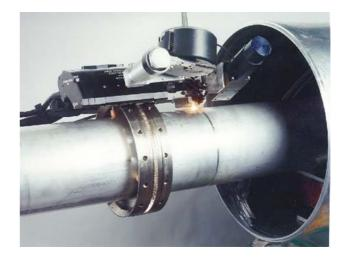
Fig. 2: Orbital welding of the conductor
